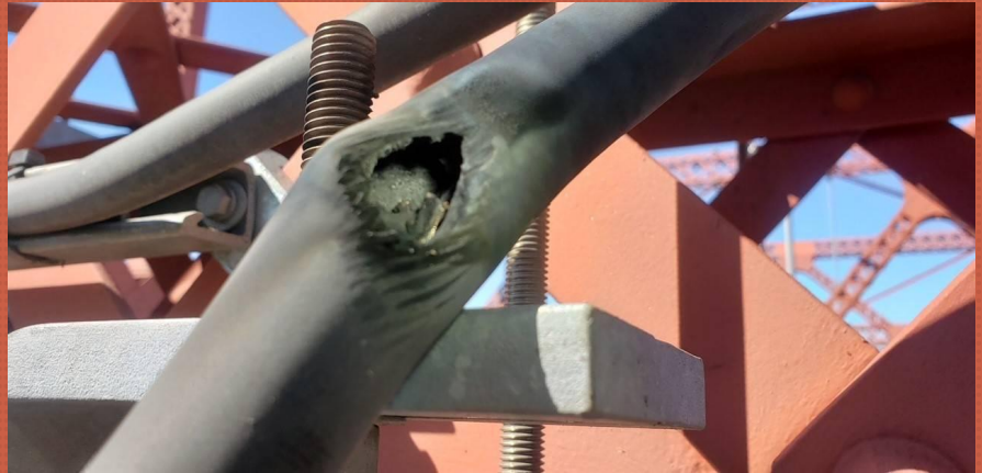
Portland Streetcar [@PDXStreetcar]. (2021, June 27). In case you're wondering why we're canceling service for the day, here's what the heat is doing to our power cables. https://t.co/EqbKUgCJ3K [Tweet]. Twitter. https://twitter.com/PDXStreetcar/status/1409287314870837253
